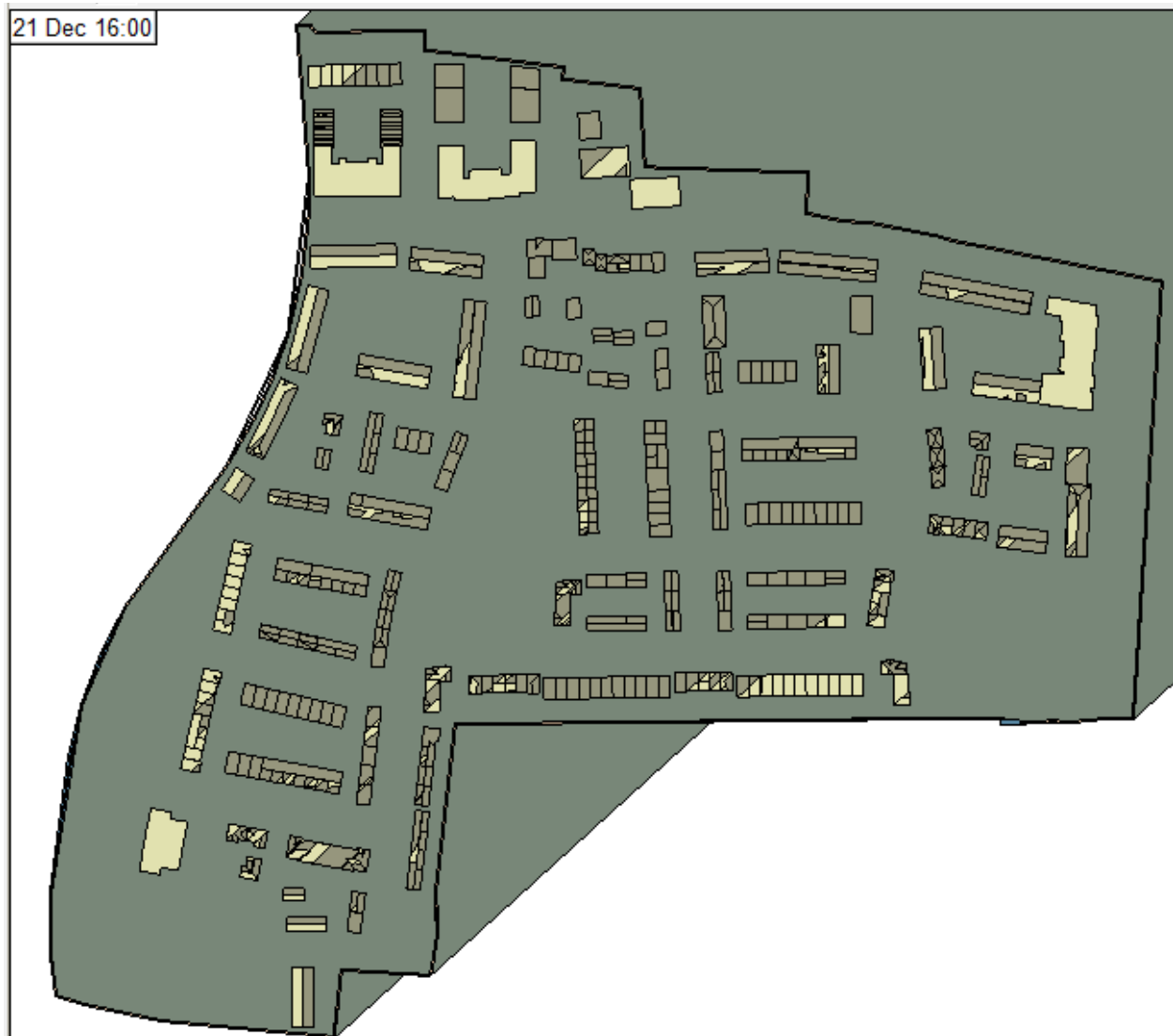
Figure 67 - Overshadowing image on December 21st at 4pm (Source IES VE model)
