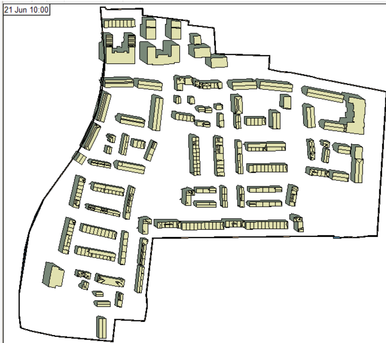
Figure 49 - Overshadowing image on June 21st at 10am (Source IES VE model)
