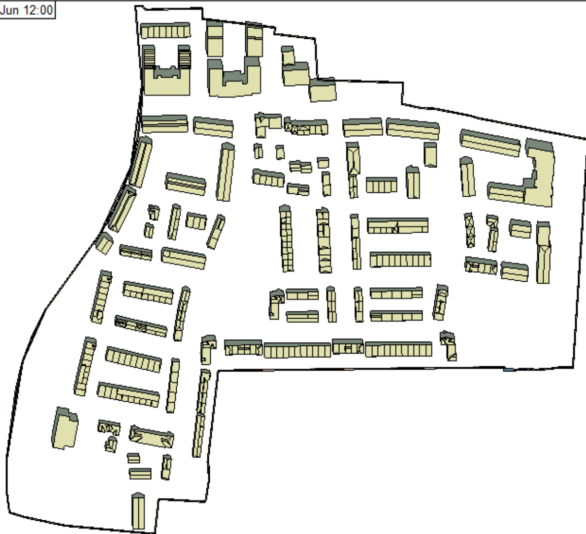
Figure 51 - Overshadowing image on June 21st at 12pm (Source IES VE model)
