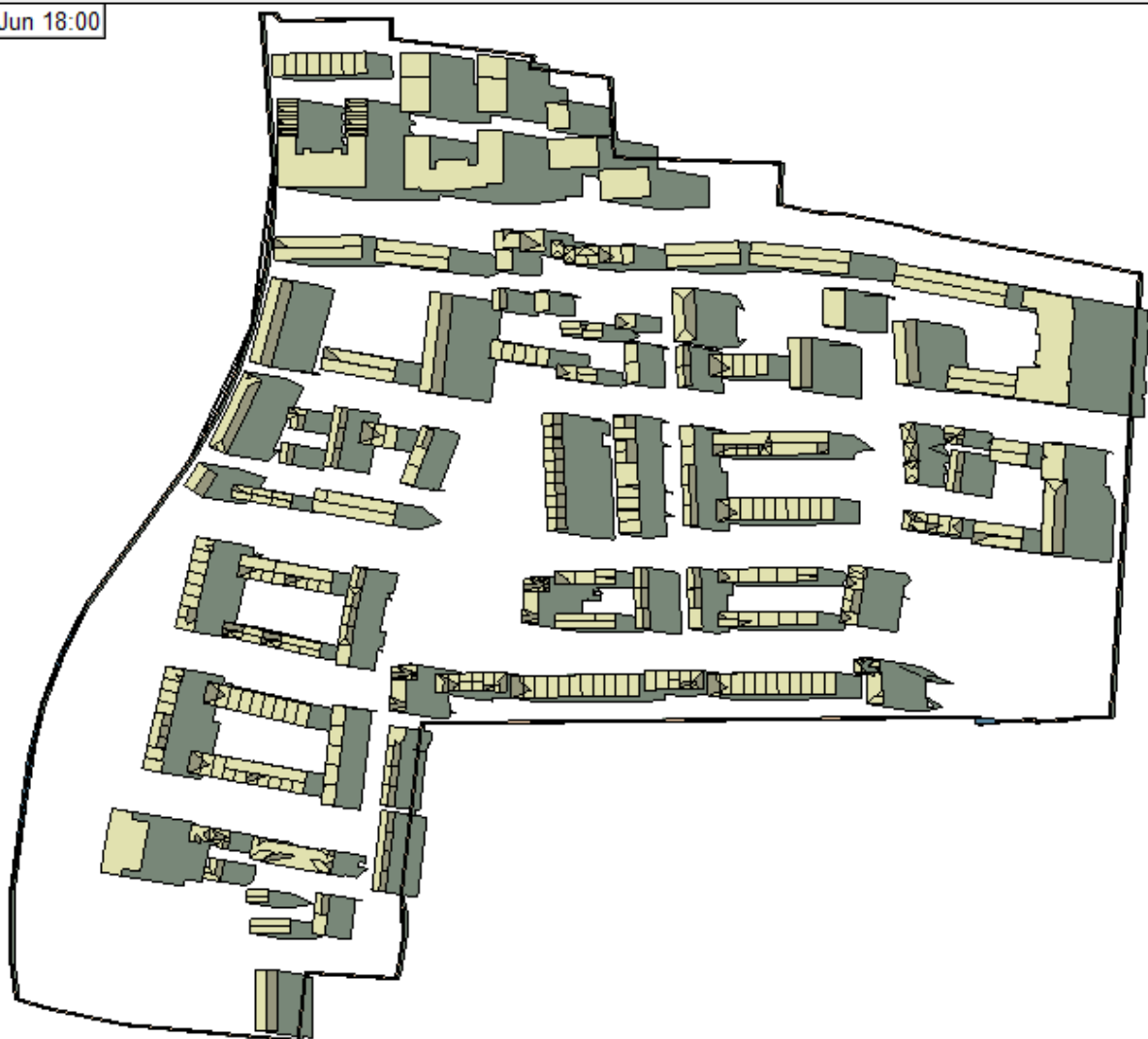
Figure 57 - Overshadowing image on June 21st at 6pm (Source IES VE model)
