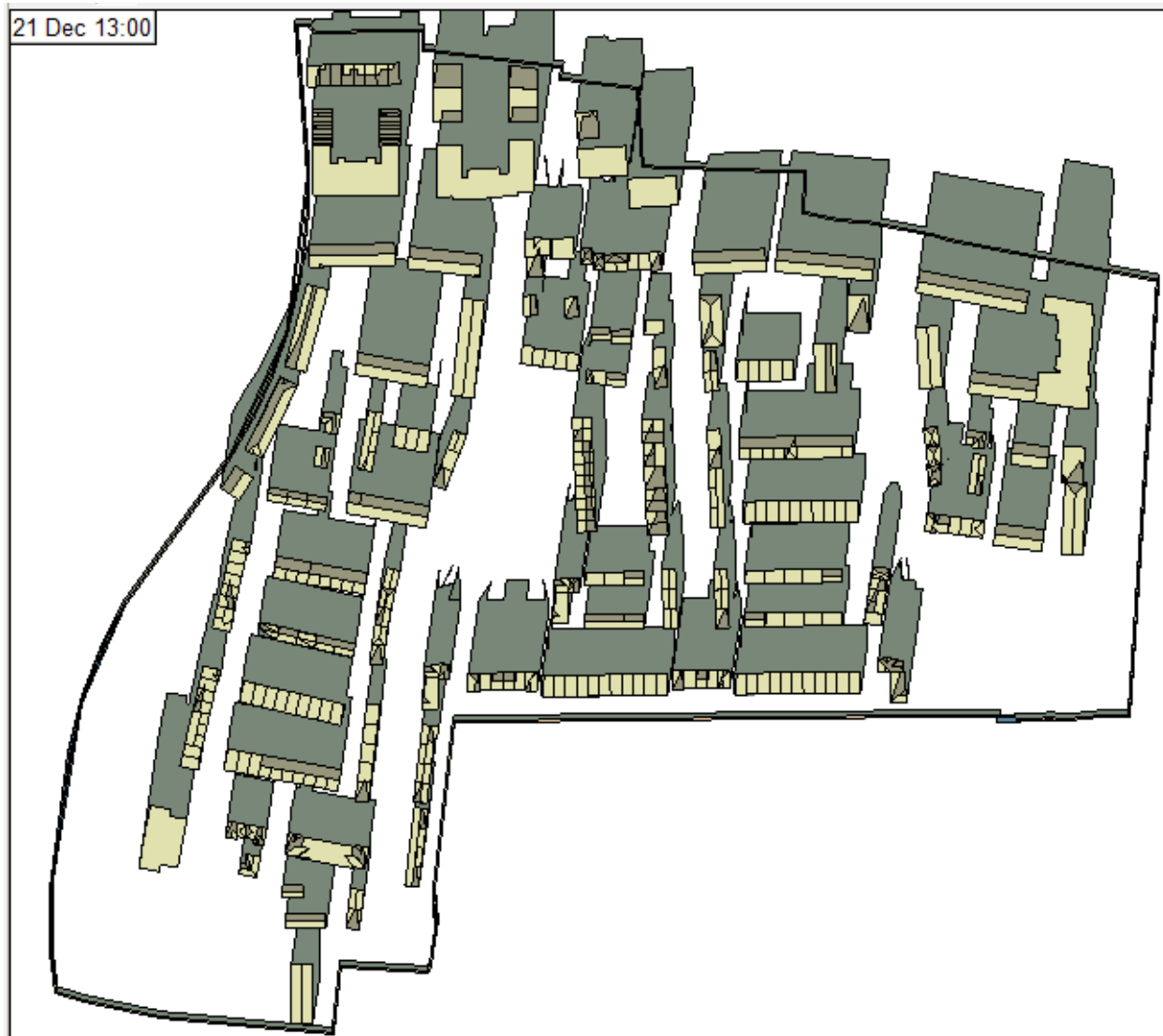
Figure 64 - Overshadowing image on December 21st at 1pm (Source IES VE model)
