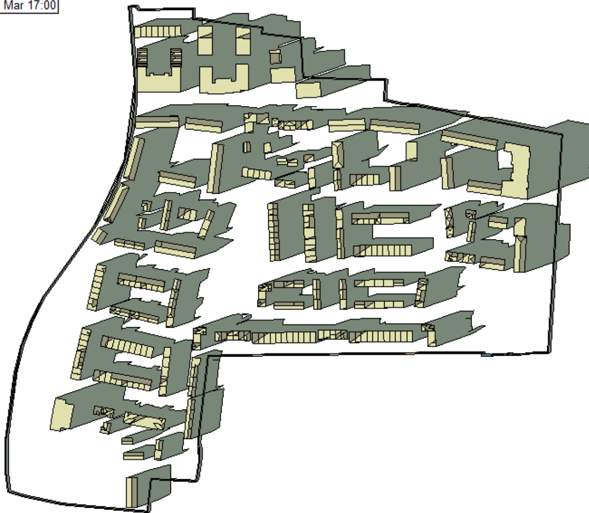
Figure 44 – Overshadowing image on March 21 st at 5pm (Source IES VE model)
