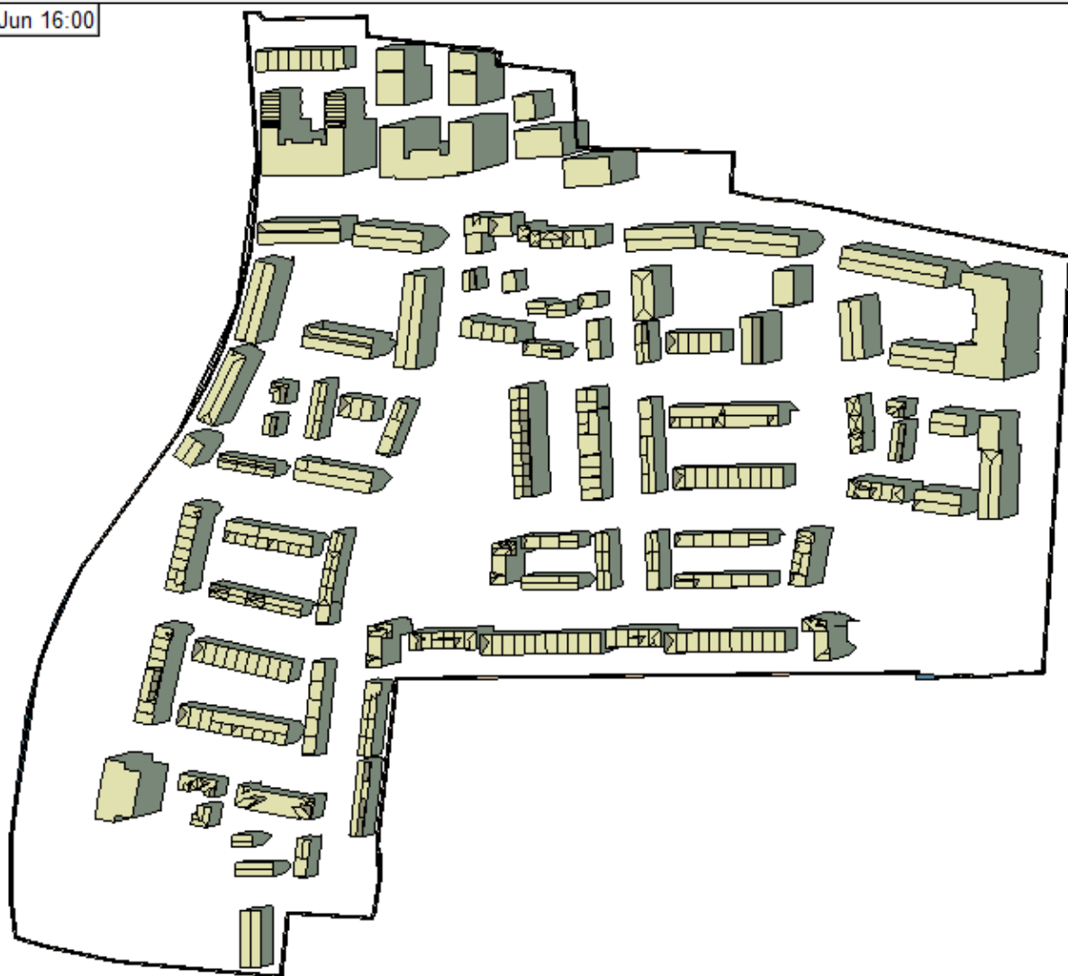
Figure 55 - Overshadowing image on June 21st at 4pm (Source IES VE model)
