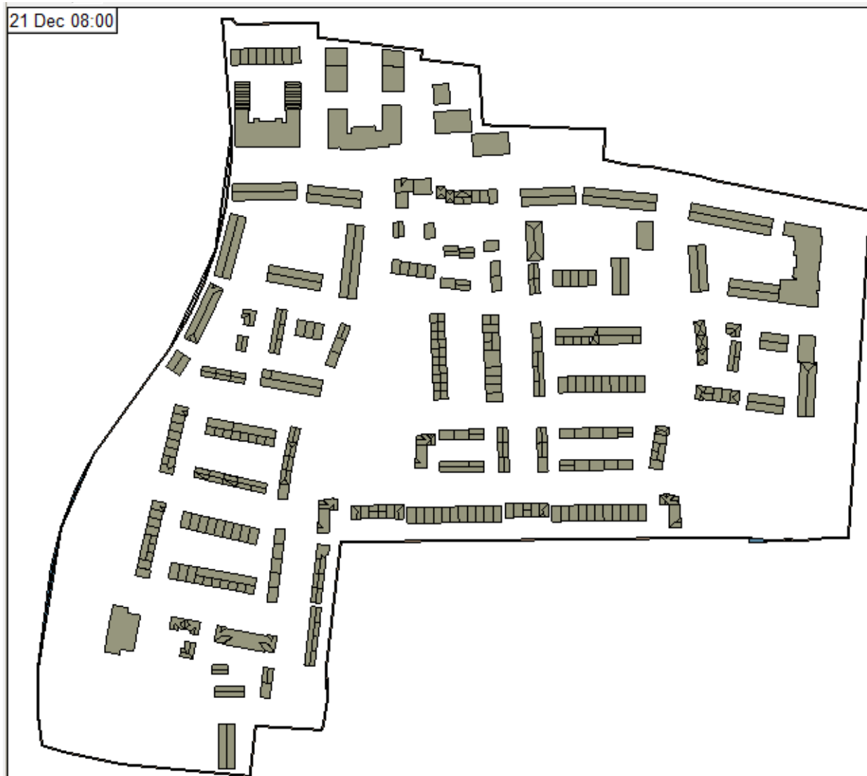
Figure 59 - Overshadowing image on December 21st at 8am (Source IES VE model)
