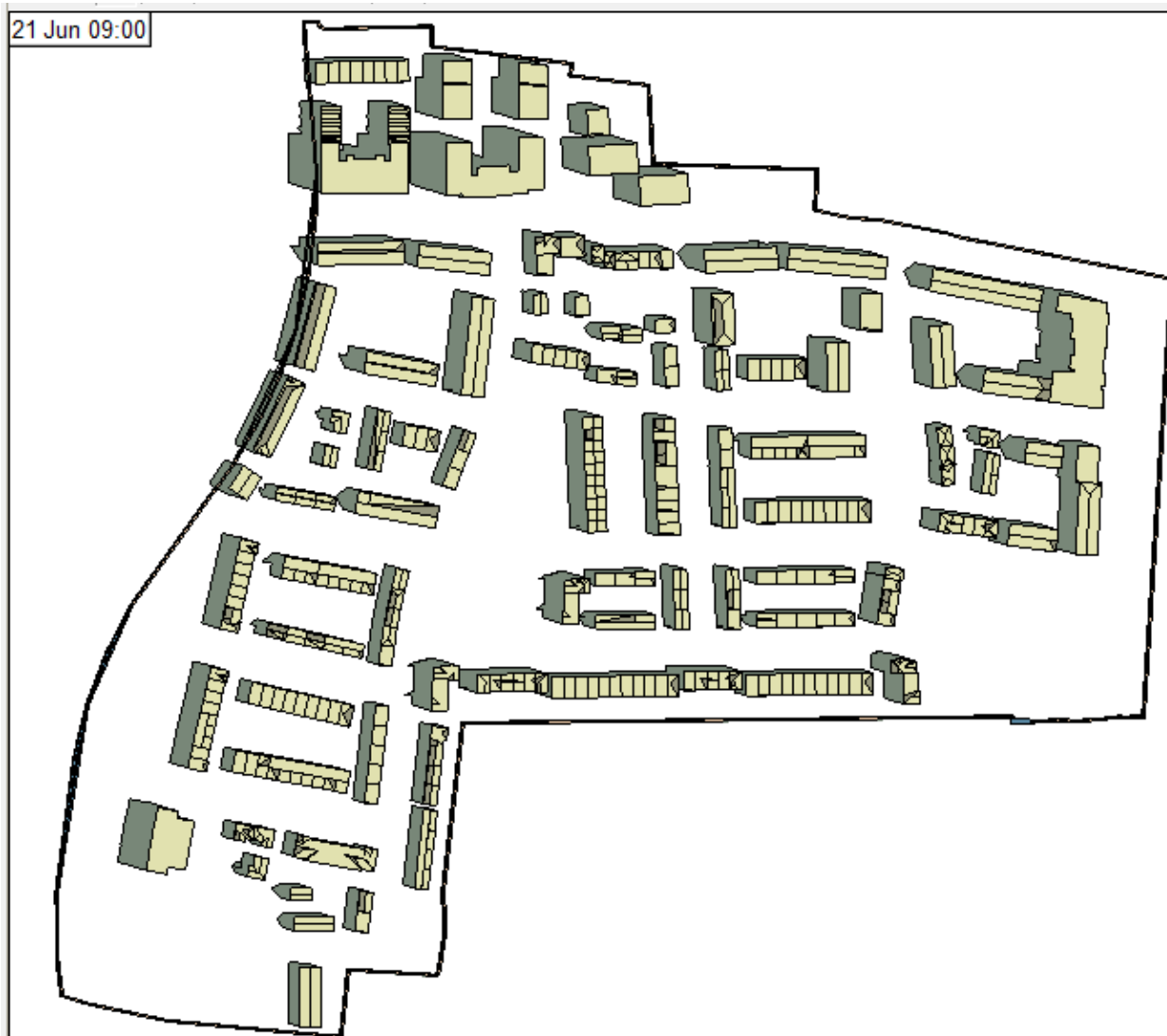
Figure 48 – Overshadowing image on June 21 st at 9am (Source IES VE model)
