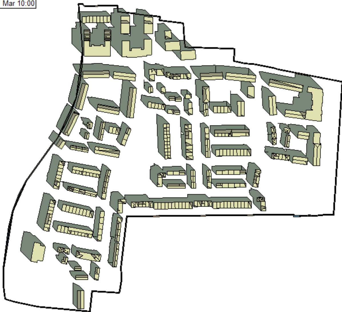
Figure 37 – Overshadowing image on March 21 st at 10am (Source IES VE model)
