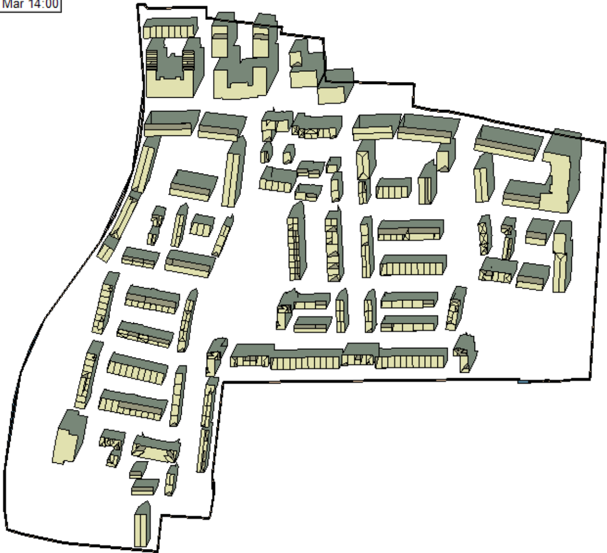
Figure 41 – Overshadowing image on March 21 st at 2pm (Source IES VE model)
