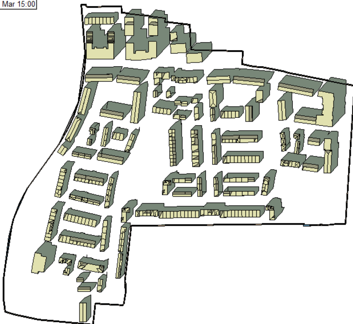
Figure 42 – Overshadowing image on March 21 st at 3pm (Source IES VE model)
