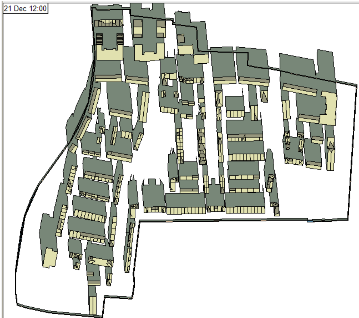
Figure 63 - Overshadowing image on December 21st at 12pm (Source IES VE model)
