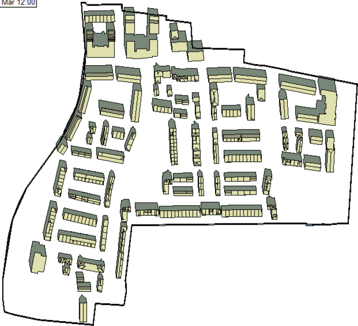
Figure 39 – Overshadowing image on March 21 st at 12pm (Source IES VE model)
