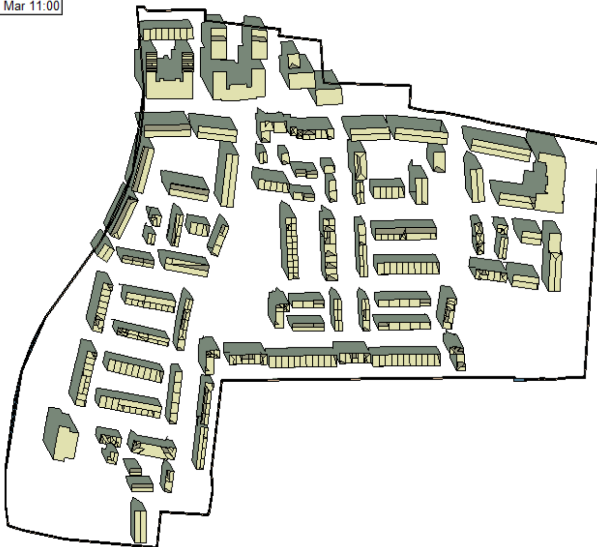
Figure 38 – Overshadowing image on March 21 st at 11am (Source IES VE model)
