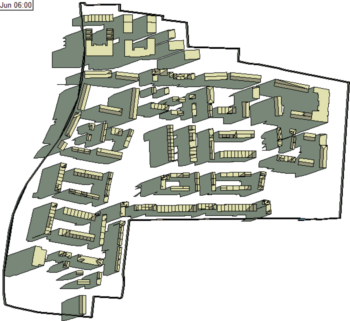
Figure 45 – Overshadowing image on June 21 st at 6am (Source IES VE model)
