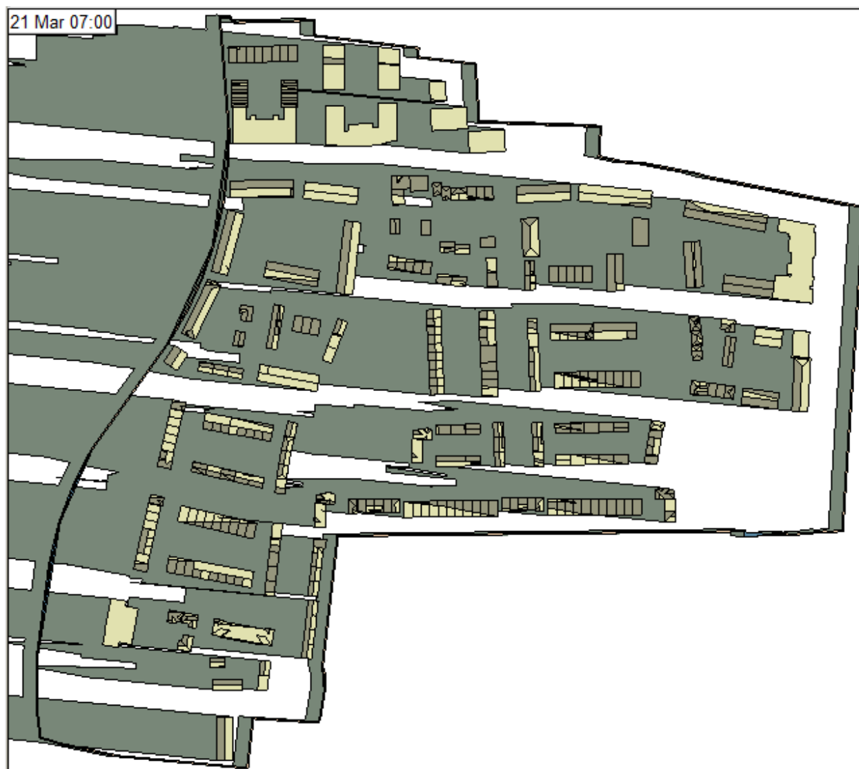
Figure 34 – Overshadowing image on March 21 st at 7am (Source IES VE model)
