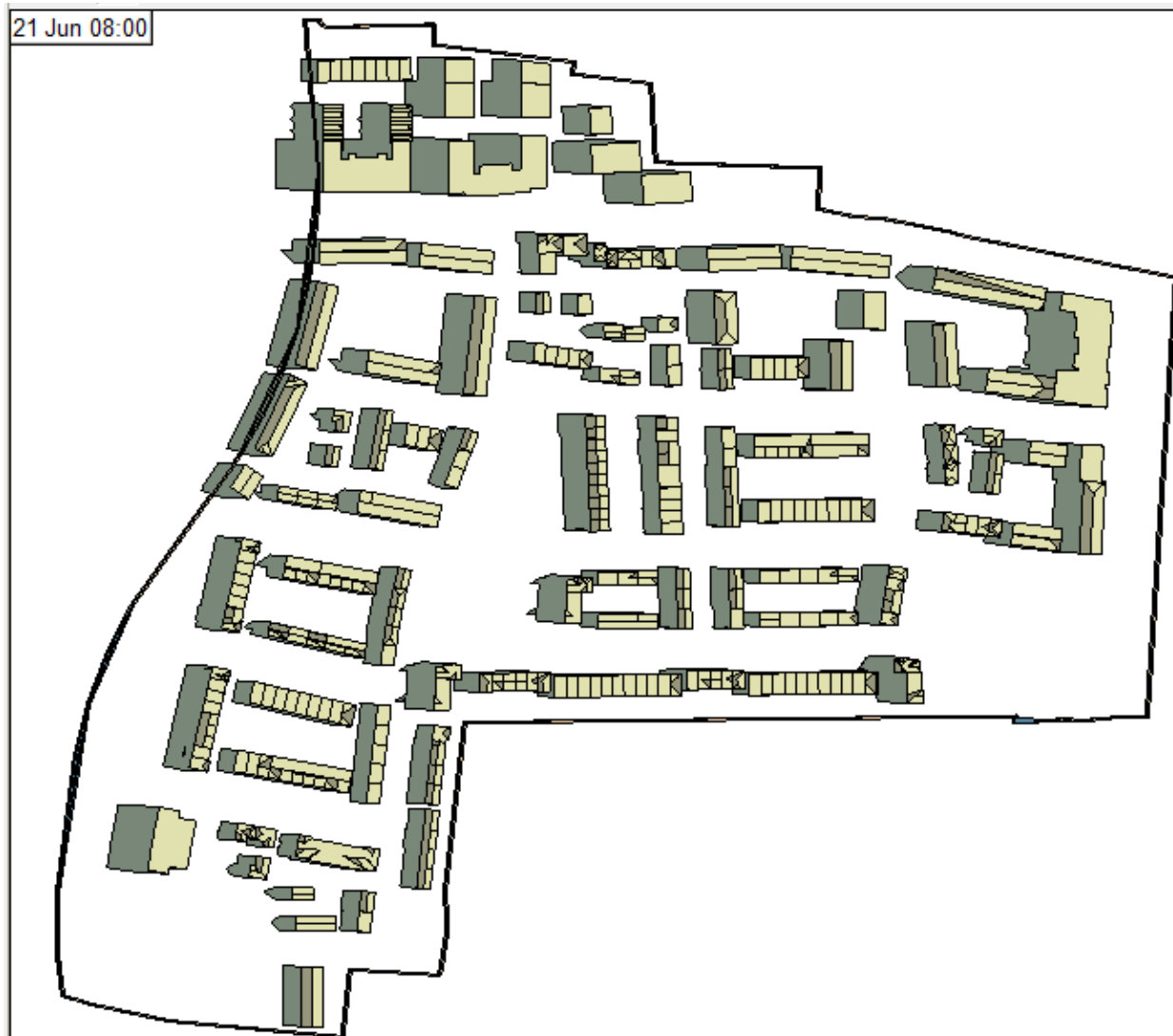
Figure 47 – Overshadowing image on June 21 st at 8am (Source IES VE model)
