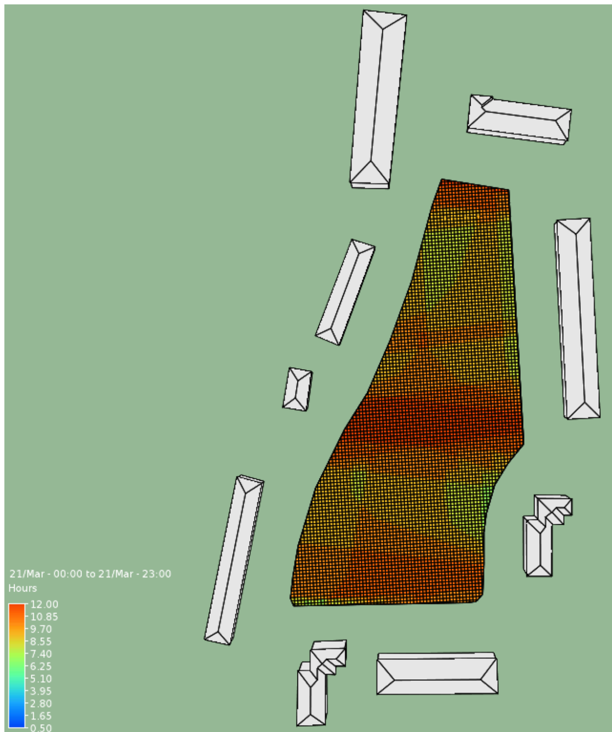
Figure 29 - Sunlight to Central Park ( K ) – More than 50% > 2 hours (Source IES VE SunCast)
