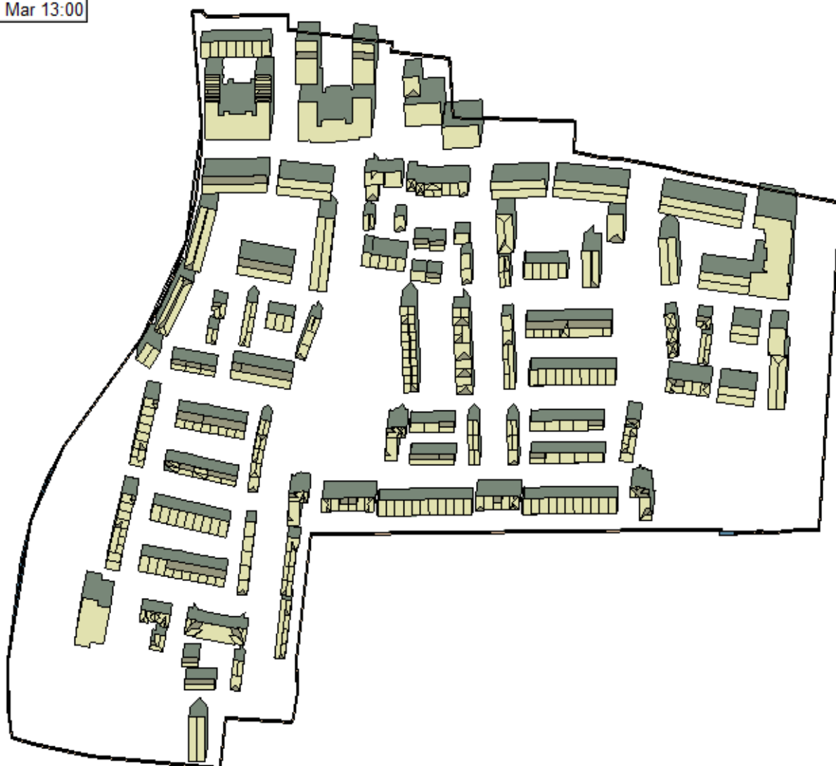
Figure 40 – Overshadowing image on March 21 st at 1pm (Source IES VE model)
