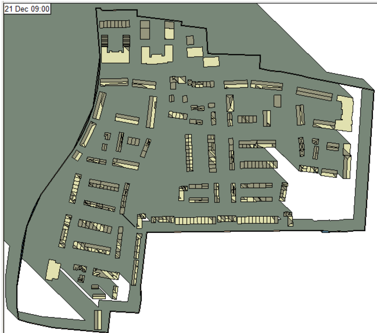
Figure 60 - Overshadowing image on December 21st at 9am (Source IES VE model)
