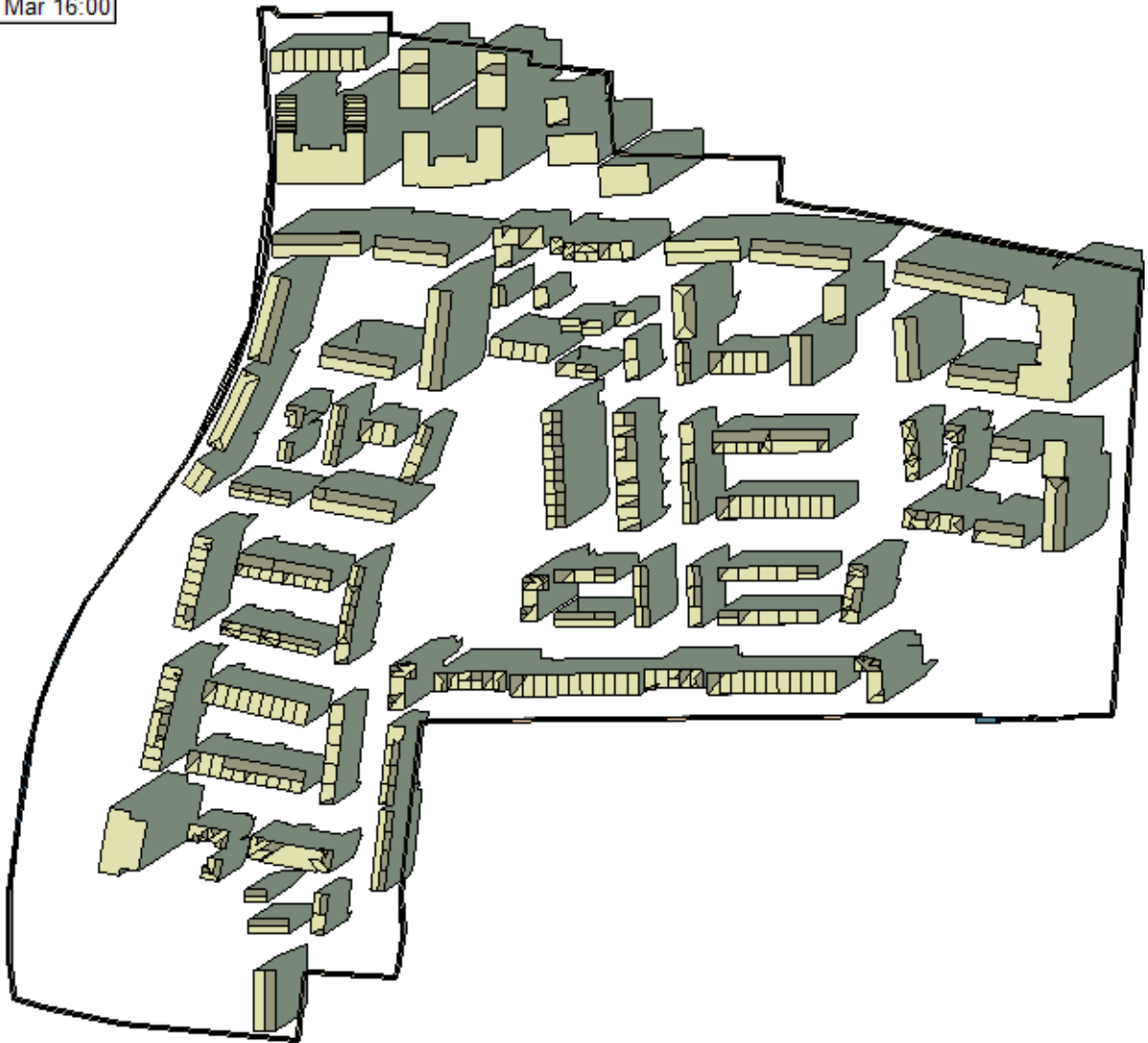
Figure 43 – Overshadowing image on March 21 st at 4pm (Source IES VE model)
