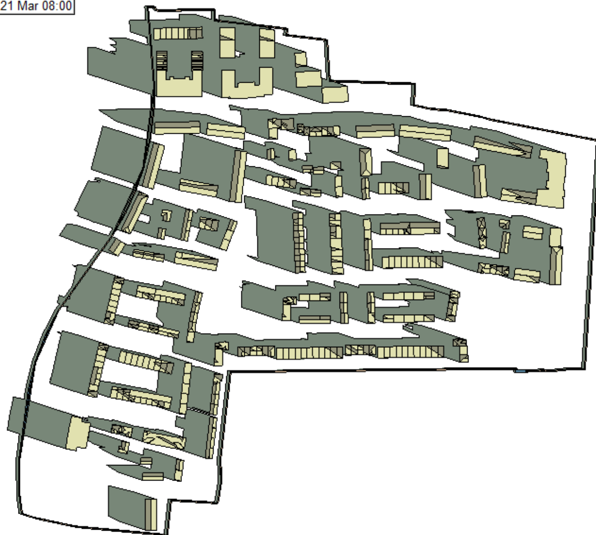
Figure 35 –Overshadowing image on March 21 st at 8am (Source IES VE model)
