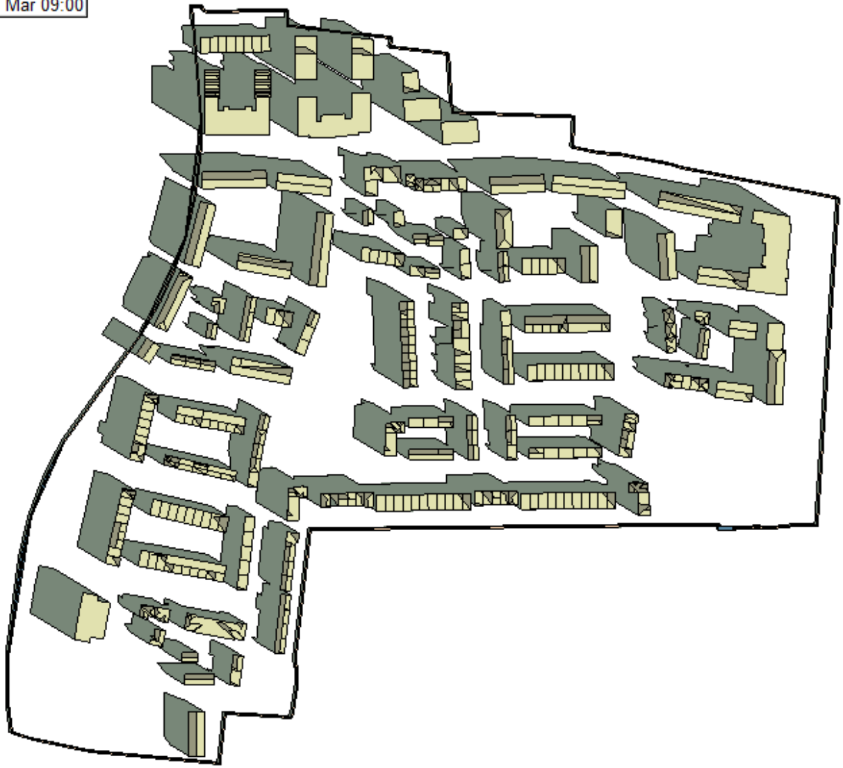
Figure 36 - Overshadowing image on March 21 st at 9am (Source IES VE model)
