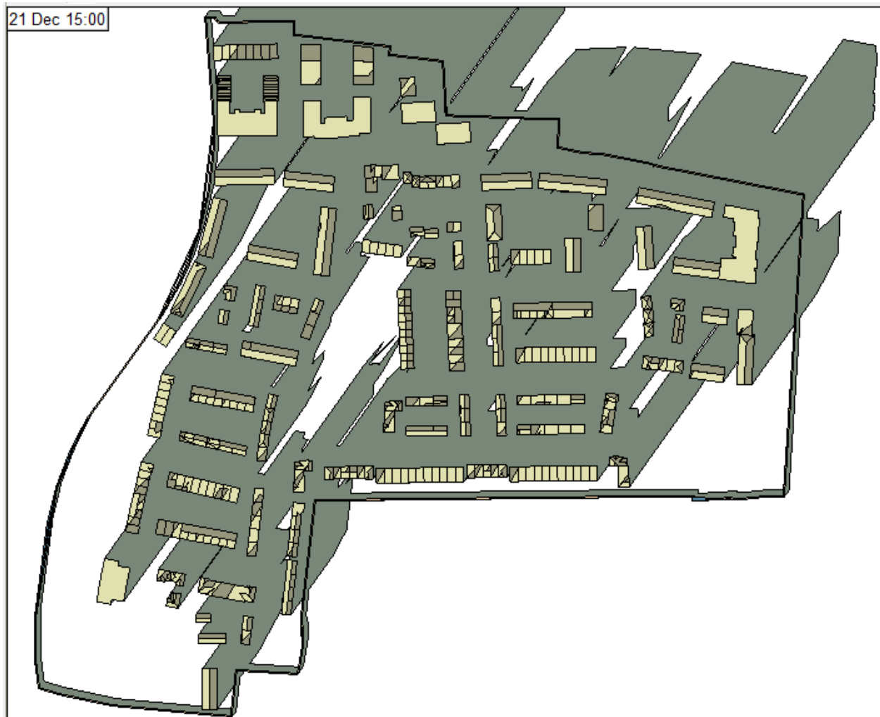
Figure 66 - Overshadowing image on December 21st at 3pm (Source IES VE model)
