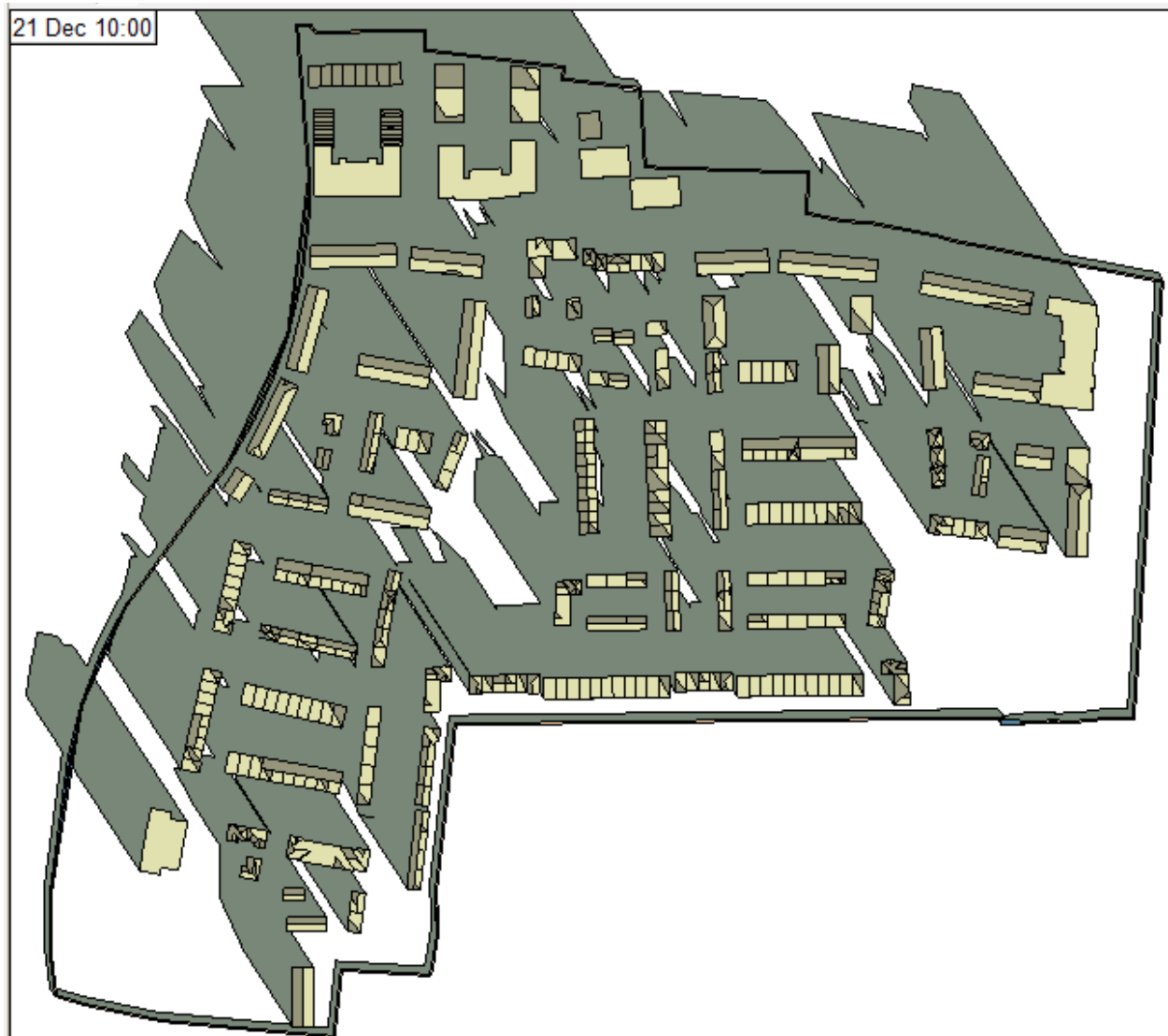
Figure 61 - Overshadowing image on December 21st at 10am (Source IES VE model)
