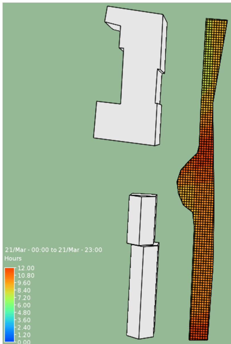
Figure 27 - Sunlight to Pocket Park (I) – More than 50% > 2 hours (Source IES VE SunCast)
