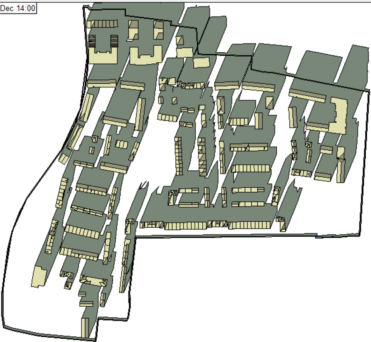
Figure 65 - Overshadowing image on December 21st at 2pm (Source IES VE model)
