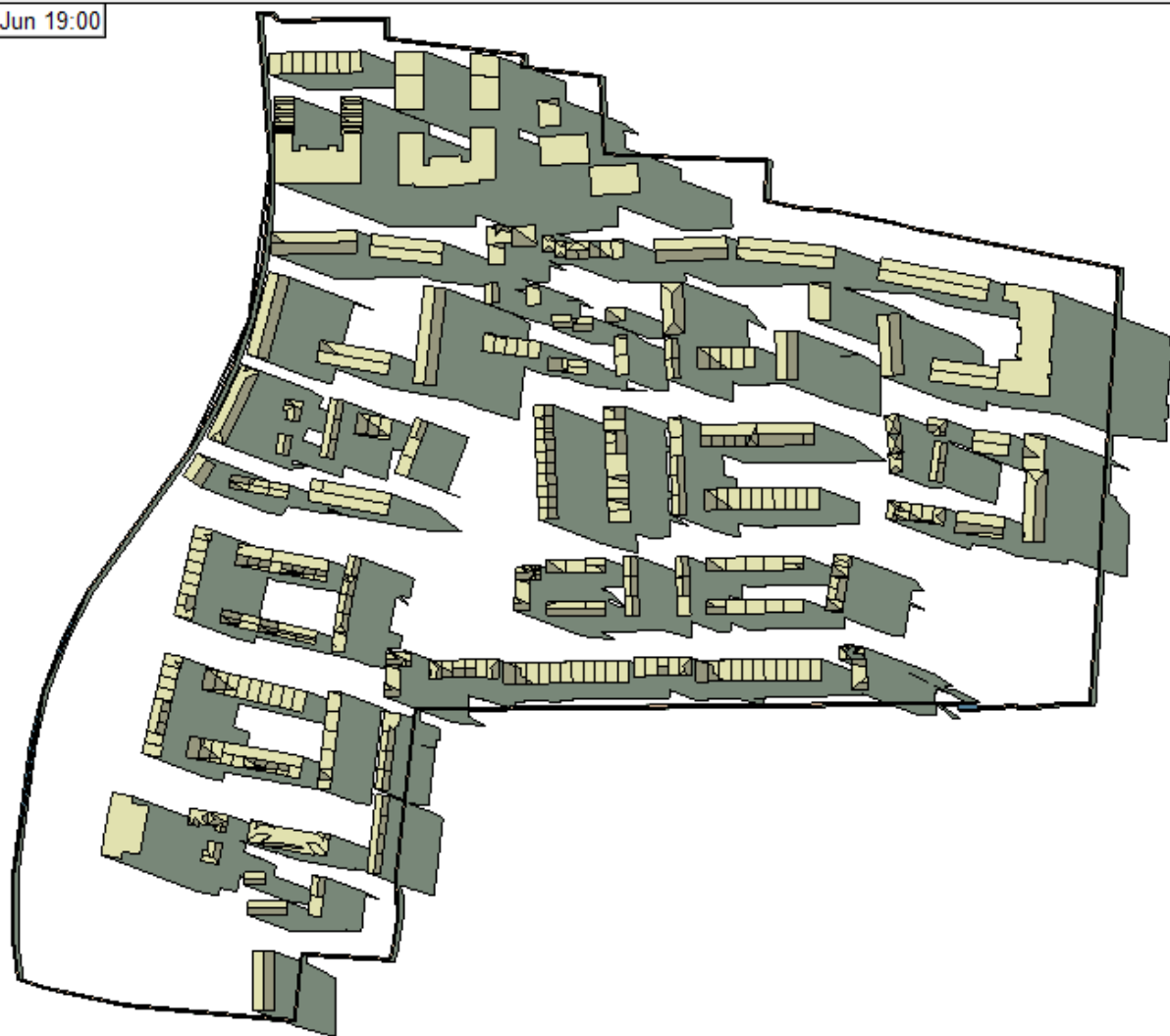
Figure 58 - Overshadowing image on June 21st at 7pm (Source IES VE model)
