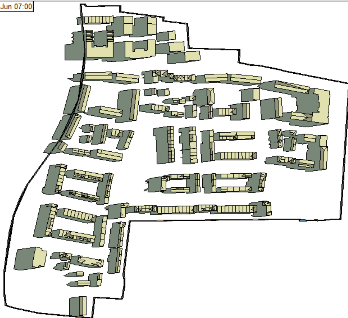
Figure 46 – Overshadowing image on June 21 st at 7am (Source IES VE model)
