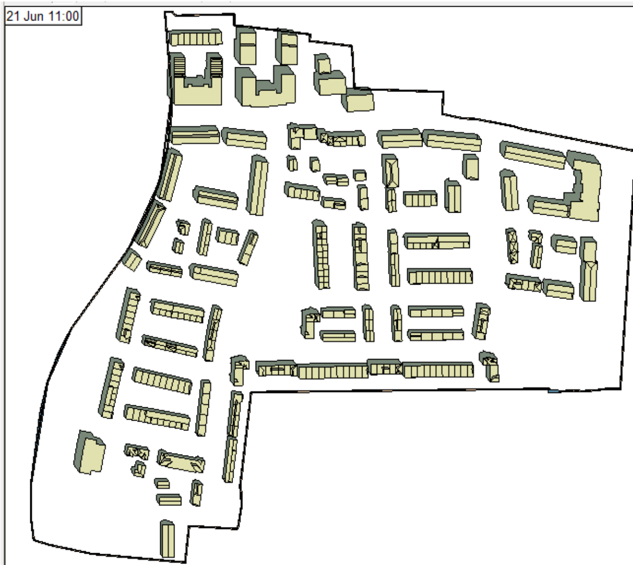
Figure 50 - Overshadowing image on June 21st at 11am (Source IES VE model)
