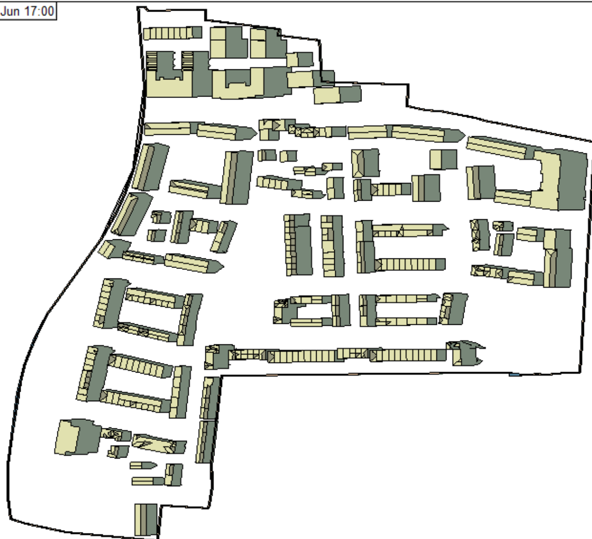
Figure 56 - Overshadowing image on June 21st at 5pm (Source IES VE model)
