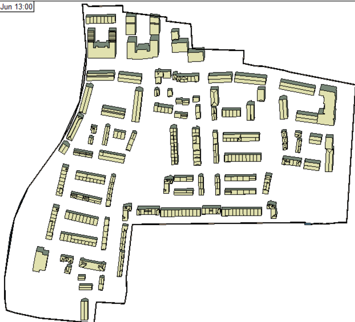
Figure 52 - Overshadowing image on June 21st at 1pm (Source IES VE model)
